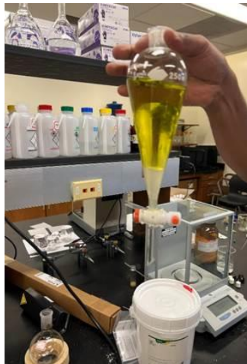
Separation of the top organic phase containing the carotenoid from the aqueous phase at the bottom.
